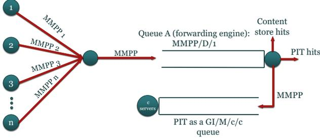
Fig. 2. Traffic flow in a router
