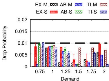
Fig. 11. Effect of demand on drop probability. The horizontal bars denote the value of  $\epsilon$ .
